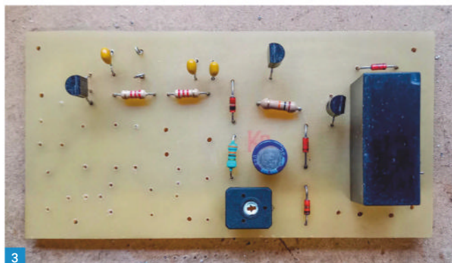
Fig. 3: Changeover board with Semi-break-in parts fitted. Fig. 4: Completed Changeover & Sidetone Board. Fig. 5: The completed RIT pot. Fig. 6: Part of VFO circuit with RIT parts C1 & D1 fitted.
