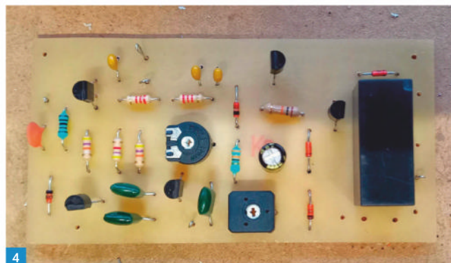
Fig. 3: Changeover board with Semi-break-in parts fitted. Fig. 4: Completed Changeover & Sidetone Board. Fig. 5: The completed RIT pot. Fig. 6: Part of VFO circuit with RIT parts C1 & D1 fitted.
