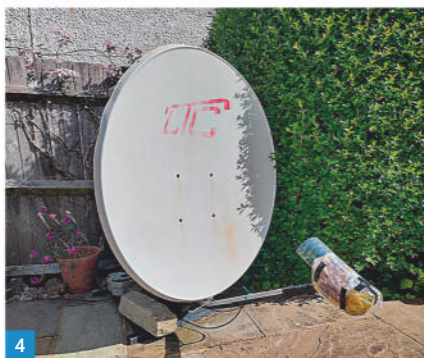
Fig. 4: A 1.1m dish and low noise block receive and transmit DATV to the geostationary QO100 satellite. Fig. 5: A 30ft crank-up mast carries a range of antennas for use on 4m, 2m and 70cm. Fig. 6: Martin (right) in his first band 'Group 36' in 1977. Fig. 7: Flying days – on route to the Channel Islands. Martin is on the right. Fig. 8: An 'extra' (left) in the feature film Cockneys vs Zombies released in 2012.
