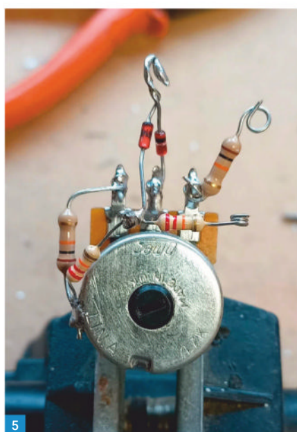
Fig. 3: Changeover board with Semi-break-in parts fitted. Fig. 4: Completed Changeover & Sidetone Board. Fig. 5: The completed RIT pot. Fig. 6: Part of VFO circuit with RIT parts C1 & D1 fitted.
